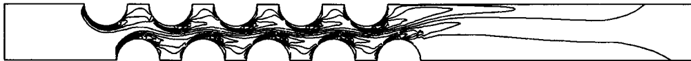
Figure 5(d). Isovorticity lines of \zeta' = (\zeta - \zeta_{\min}) / (\zeta_{\max} - \zeta_{\min}) with \Delta \zeta' = 0.05 for the five-row-deep bundle of cylinders in Figure 1(a); Re = 200 , P/D = 1.5
