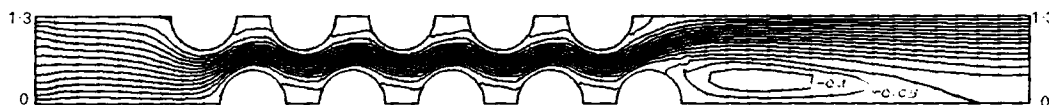
Figure 5(a). Streamlines \psi with \Delta\psi = 0.1 except for the vortex region behind the last row ( \Delta\psi = 0.05 ) for the equilateral triangular arrangement in Figure 1(a) with Re = 100 and P/D = 1.5
