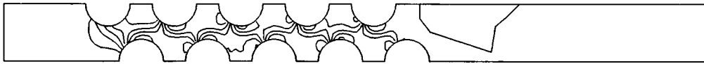
Figure 5(c). Isobars of p' = (p - p_{\min}) / (p_{\max} - p_{\min}) with \Delta p' = 0.05 for the five-row deep bundle of cylinders in Figure 1(a); Re = 200 , P/D = 1.5
